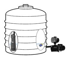
To prevent a pump from starting below a certain water level. This option is preferable to relying on in-built dry run protections
